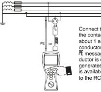
Connect the meters as shown in the figure, touch the contact electrode with your finger and wait about 1 second. When the voltage on the **PE** conductor is detected, the instrument displays the **PE** message (error in the installation, the PE conductor is connected to the phase conductor) and generates a continuous audio signal. This option is available for all measurement functions related to the RCD's and fault loop, except for **Z**L-N,L-L.
