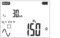
Protective conductor resistance for RCD -R<sub>F</sub>
