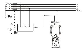
Checking the effectiveness of protection against electric shock of the equipment casing for: a) TN mains b) TT mains.
