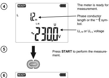
Read the main result: the fault loop impedance  $Z_S$  and the mains voltage during the measurement.
